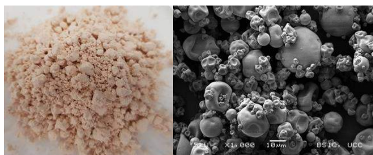
Figure 22. Scanning electron microscope of lentil protein isolate, isolated by isoelectric precipitation.
